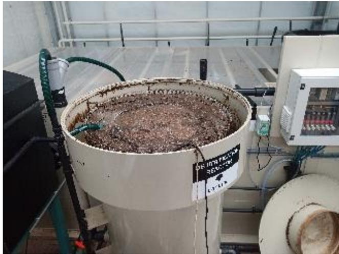
*Figure 4: initial reactor configurations showed an excess of solids buildup at the top. This provided excellent solids capture, but little NO<sub>3</sub> removal.*
